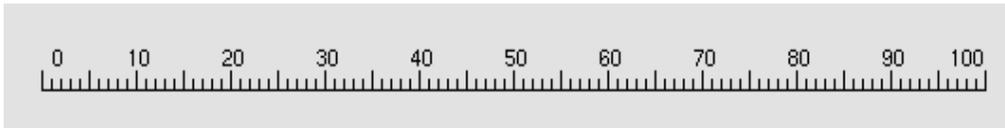
Axis shows the range for a curve or bar in x or y direction. There are two variants of Axis, one with static min and max values, and one with dynamic min and max values, where min and max are connected to signals in the database. For a dynamic Axis object, the values of Lines, LongQuotient, ValueQuotient and Format are calculated automatically in runtime.
